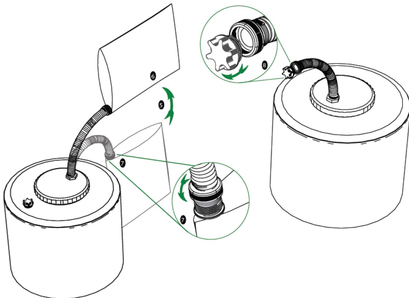
5. Lift bag to allow product to dispense thru RDS into mixing tank.
